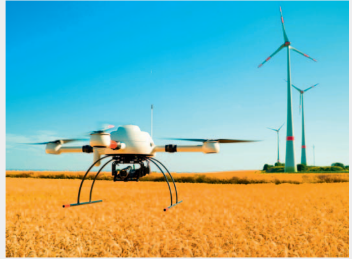
Figure 2. Microdrone md4-1000 with camera system during flight operation.
