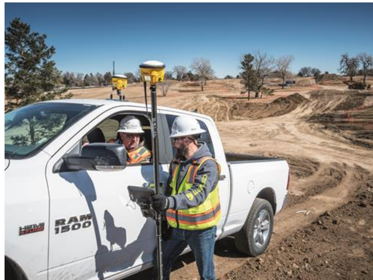
Trimble's TSC7 Controller with its SPS986 mode
