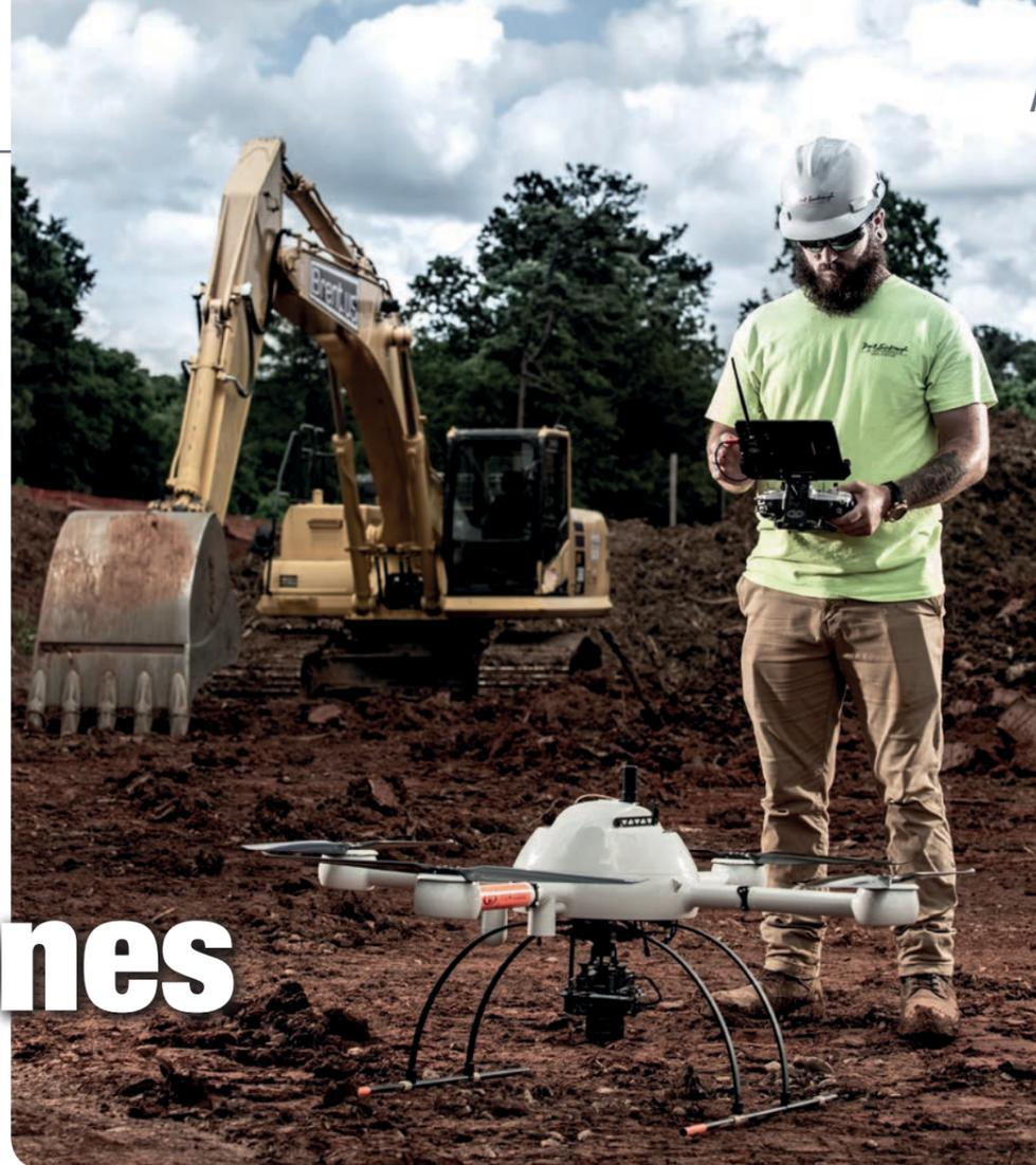
All components are precisely integrated to perform together. This allows for real-time monitoring since the flight control can run fully automatically. The system is also equipped with the Applanix APX-20 to deliver the best achievable positional accuracy. Recording data requires less overlap to achieve the required accuracy levels. The solution also includes mdLiDAR Processing Software, tailored specifically to the mdLiDAR product line for creating corrected and accurate 3D point clouds.
